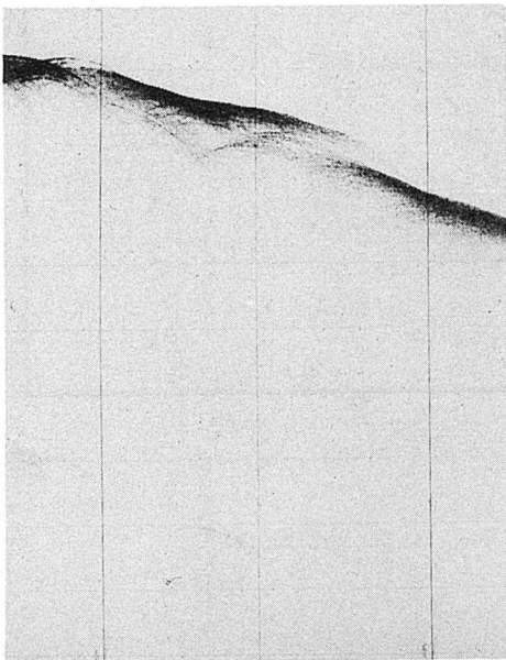
Fig.3. Echosounder reflection profile in E part of the dumpsite. Vertical range 4124-4875 m. Vertical scale exaggerated 50 \times .
