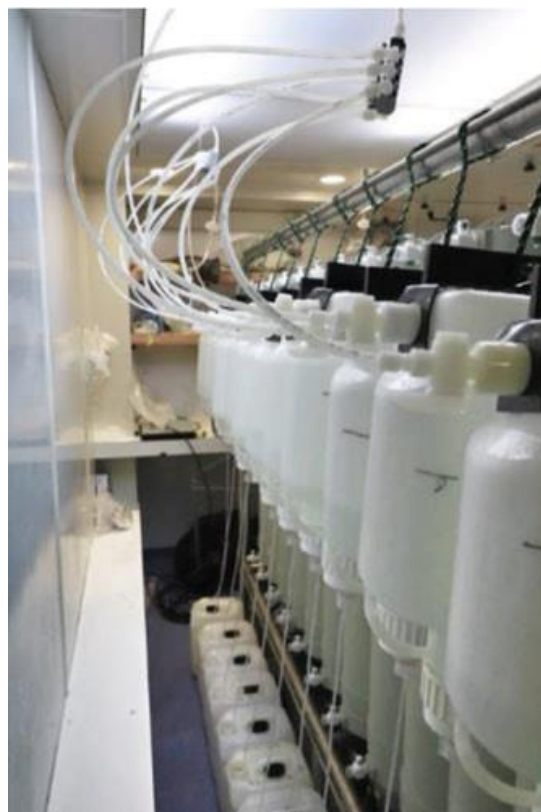
Fig. 3.12 Photograph of a custom-built off-line particulate trace metal set-up (photograph credit: Mathijs van Manen, NIOZ, Netherlands). For the off-line particulate trace metal set-up, water samples were collected from the bottle samplers right after recovery into secondary containers to decrease between-cast turnaround time (Cutter et al. 2017)
