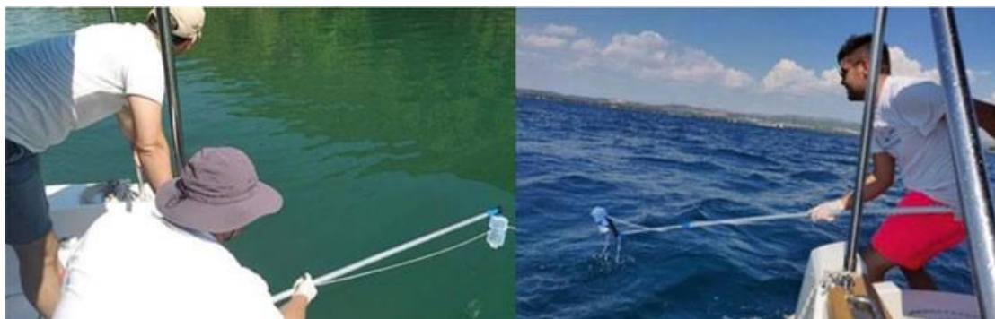
Fig. 3.11 Photographs of a pole sampler for collecting near-surface water samples directly from the coast or from an inflatable rubber boat (photograph credit: Dario Omanović, Rudjer Boskovic Institute, Croatia)
