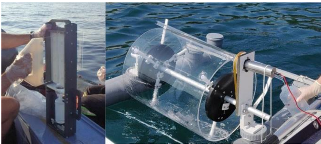
Fig. 3.10 Photographs of a sea surface microlayer (SML) plate sampler (left) (photo credit: Antonio Tovar Sánchez, ICMAN (CSIC), Spain), and a SML drum sampler prototype (right) (photograph credit: Dario Omanović, Rudjer Boskovic Institute, Croatia)
