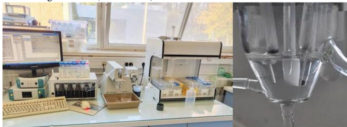
Fig. 3.24 Photograph of an automated voltammetry set-up (left) and a three-electrode voltammetric cell (right) (photograph credits: Dario Omanović, Rudjer Boskovic Institute, Croatia)
