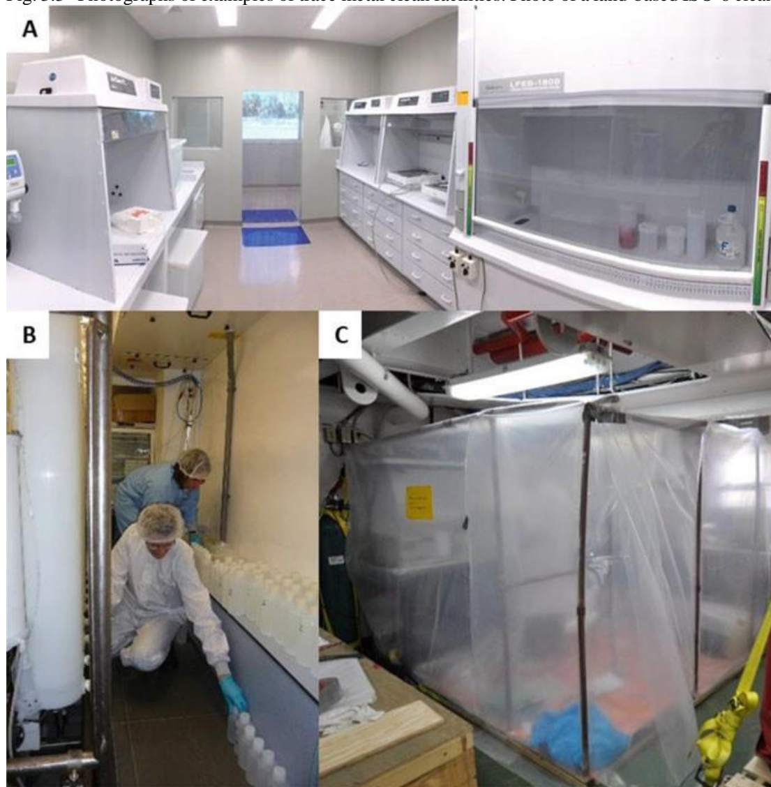
laboratory with ISO-5 laminar flow hoods (a) (photograph credit: Tim Conway, University of Florida, USA), the NIOZ trace metal clean container (b) (photograph credit: Loes Gerringa, NIOZ, Netherlands) and a trace metal clean working 'bubble' on board a research vessel (c) (photograph credit: Gert van Dijken, Stanford University, USA)
