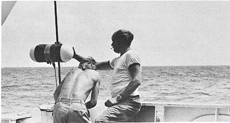
Quantum scalaire irradiantimeter.
