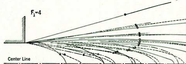
FIG. 54.—EXPERIMENTAL MEASUREMENTS OF SURFACE CONFIGURATION FOR VARIOUS FROUDE NUMBERS AND WIDTH-DEPTH RATIOS
