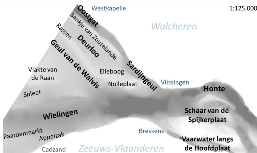
Figure 2. Bathymetry of the Scheldt mouth (1972) with the names of the major features
