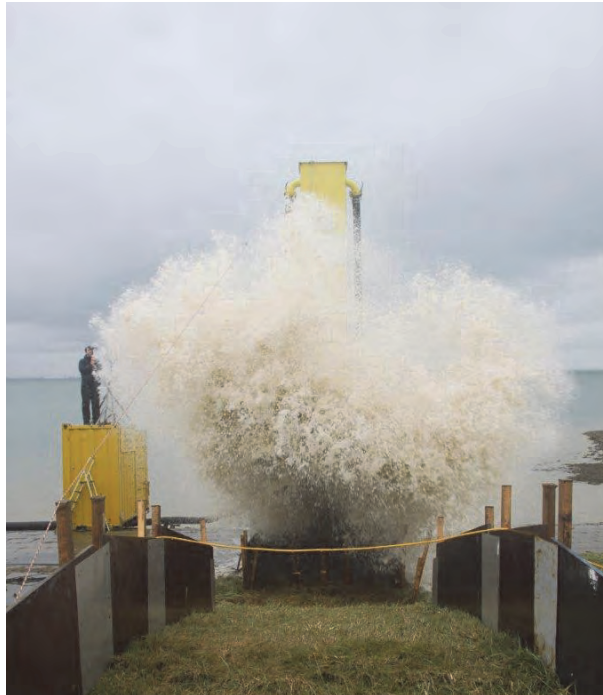
Figure 4.37 Measuring wave impacts on a 0.46 m high vertical step of a stair case, caused by run-up flows on a promenade from the wave run-up simulator
