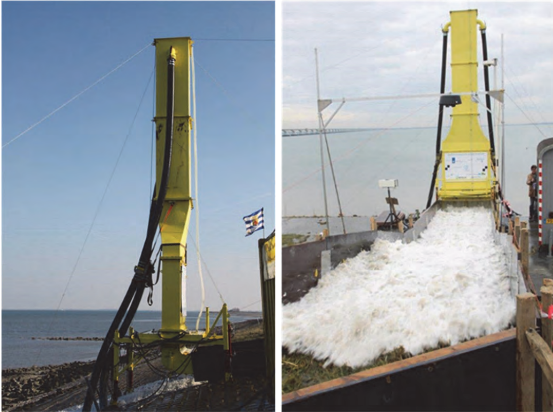
Figure 4.40 The Wave Run-up Simulator
