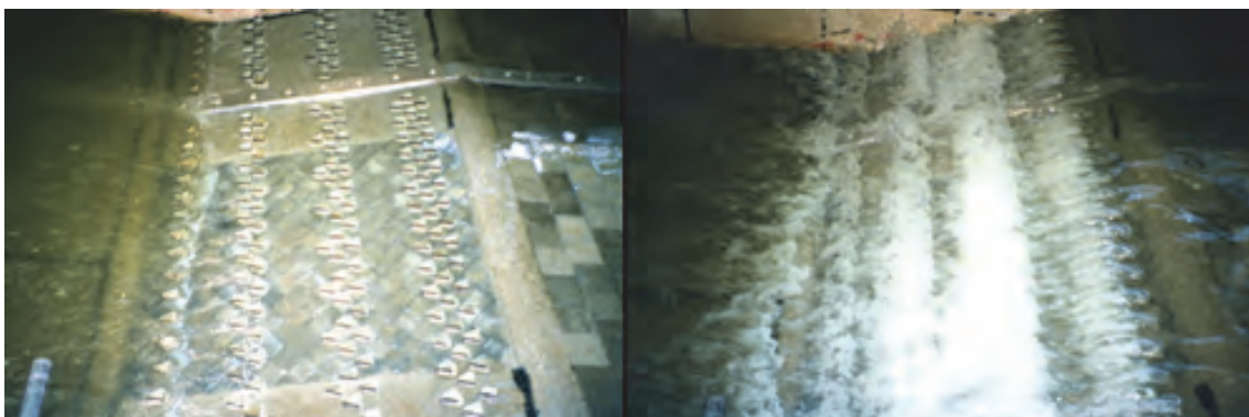
Figure 5.23: Performance of roughness elements showing the degree of turbulence
