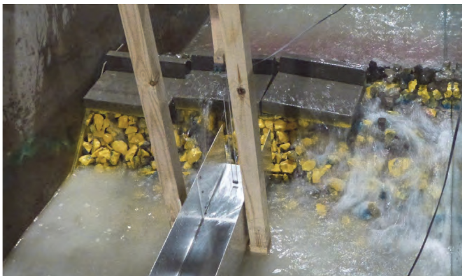
Figure 3.10: Breakwater design under overload conditions and near to complete failure
