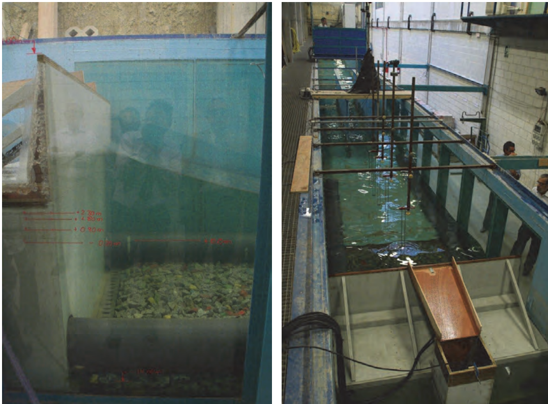
Figure 4.28: Cross-section of a vertical caisson in a wave flume (left) with the overtopping chute and tank (right). Wave flume at INHA, ES
