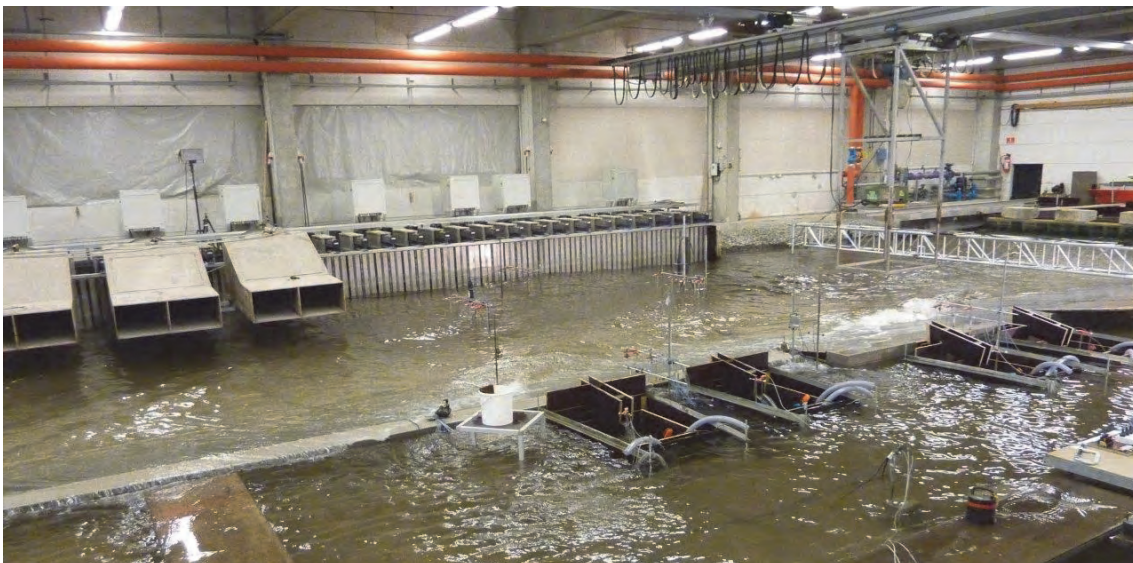
Figure 4.29: Testing wave overtopping of a dike slope 1:6 in a wave basin, including simulation of currents (from right to left). Part of the short-crested wave generator has also wind generators (upper left). Overtopping was measured in various boxes, middle right. Wave basin at DHI, DK
