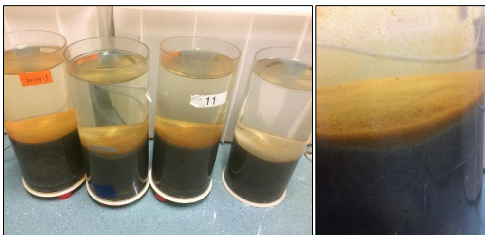
Figure 8. Photos of iron oxide formation in three PDC exposed cores next to one control core (left). A closer look at newly formed iron oxides on the sediment surface and in the water column (right).
