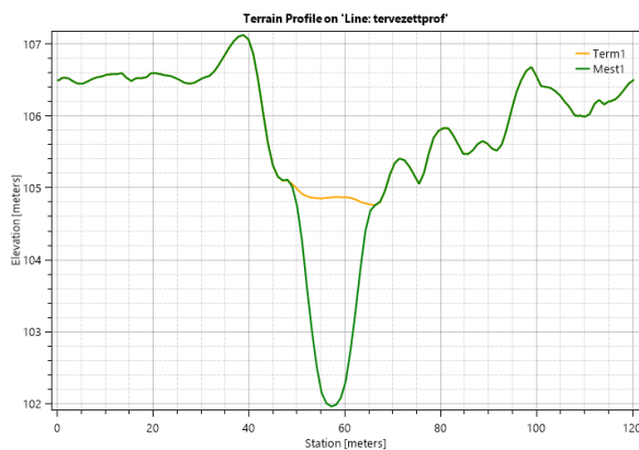
Figure 16. Natural and planned cross-profile of the flood plain channel (the cell size of the calculation grid was 1 meter).
