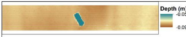
Figure 5: Initial laboratory scan of the object using SeaTek 5MHz ultrasonic transducers prior to flow.
