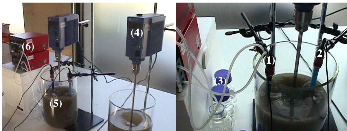
Figure 4. Photographs of the experimental set-up used for the sediment suspension simulations. (1) pH electrode; (2) temperature electrode; (3) acid/base; (4) electrical mixers; (5) reactor vessel with suspended sediment; (6) pumps for acid/base dosage.
