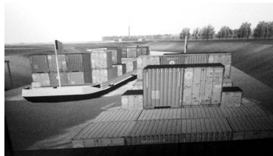
Figure 3: Passage of two class IV inland vessels on a section of the Upper-Sea Scheldt (scheme and simulation)
