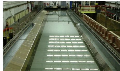
Figure 7: Graphical presentation of weight distribution (left) and four bank types in the towing tank (vertical wall, slope 1/1, 1/3 and 1/4)
