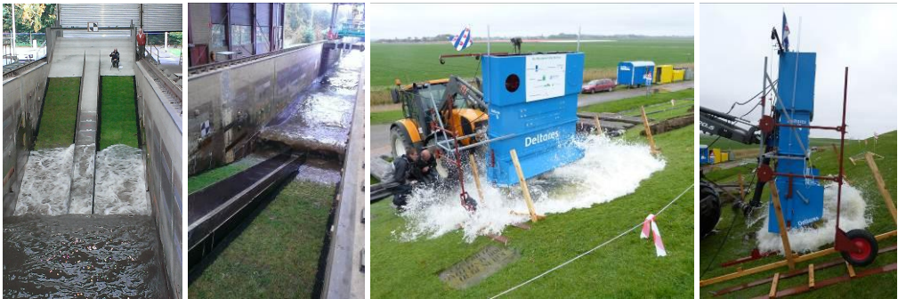
Figure 1. left: traditional testing of grass slope in a large-scale wave flume. Right: testing of grass slope with wave impact generator
