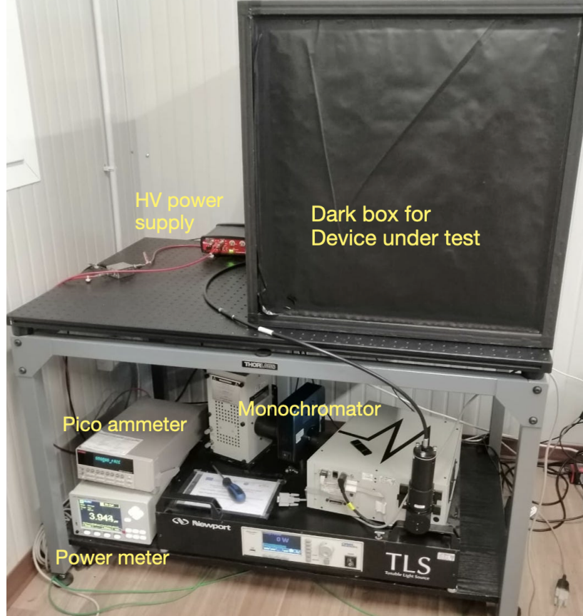
Figure 1. The test setup for photocatode scan and quantum efficiency measurements at the Capacity laboratory of the Istituto Nazionale di Fisica Nucleare (INFN) located in Caserta. The dark box contains the PMT under test and the 2D moving stage. The lower part of the picture shows the Xenon lamp, the monochromator and the electronic circuits required for the data acquisition.
