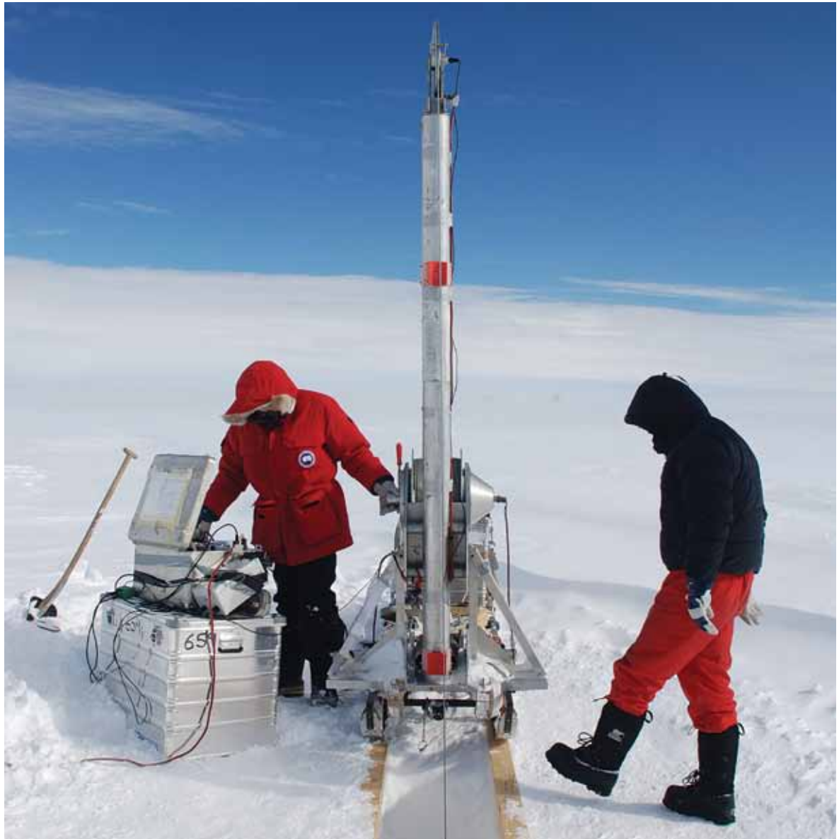
Fig. 2.4-4. Drilling a shallow ice core near the NEEM site on the Greenland Ice Sheet, July 2008. (Photo: NEEM ice core drilling project, www.neem.ku.dk, Henning Thing)
