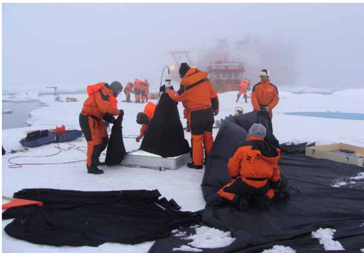
Fig.5.3-2. Optical experiment for sea ice in the summer Arctic. For comparing with winter results, an optical experiment with natural light and artificial light was undertaken during the 2008 summer cruise of Xue Long. A large area must be covered by thick black cloth for the artificial light experiment.
