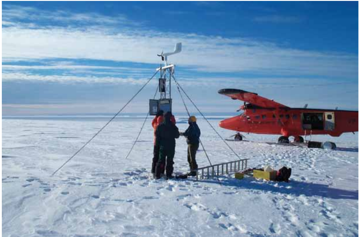
Fig. 3.5-3. Servicing the AWS at Butler Island (U.K./U.S.A.). (Photo: Jon Shanklin)
