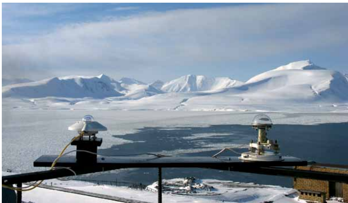
Fig. 2.1-2. Yanishevsky-Savinov (right) and Kipp and Zonen (left) pyranometers used in intercomparisons carried out at the Russian station Barentsburg (Svalbard) in April 2008. (Photo: Boris Ivanov; Ivanov et al., 2008).
