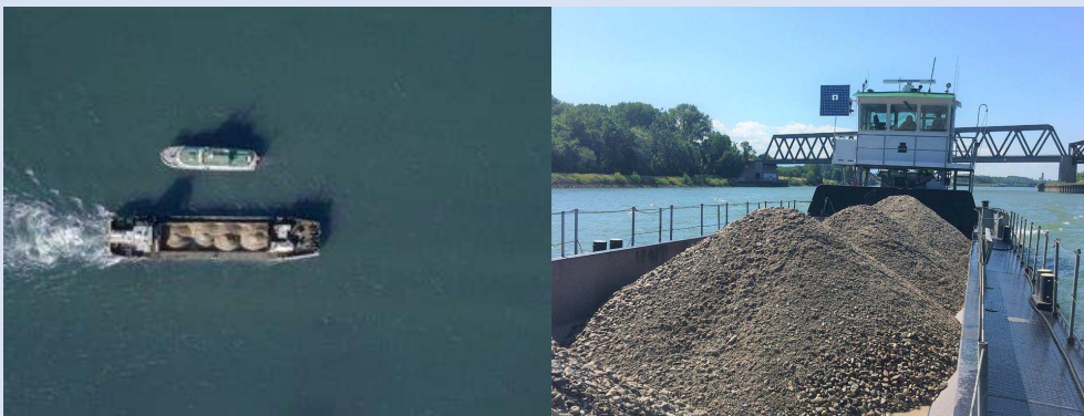
Fig.2.6: Sediment nourishment Upper Rhine (source: blubb.media GmbH)
