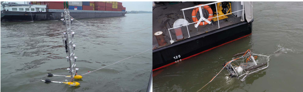
Figure 2.5: Monitoring suspended matter and bedload at the Lower Rhine". Source, Copyright: BAW, Karlsruhe (Federal Waterways Engineering and Research Institute)
