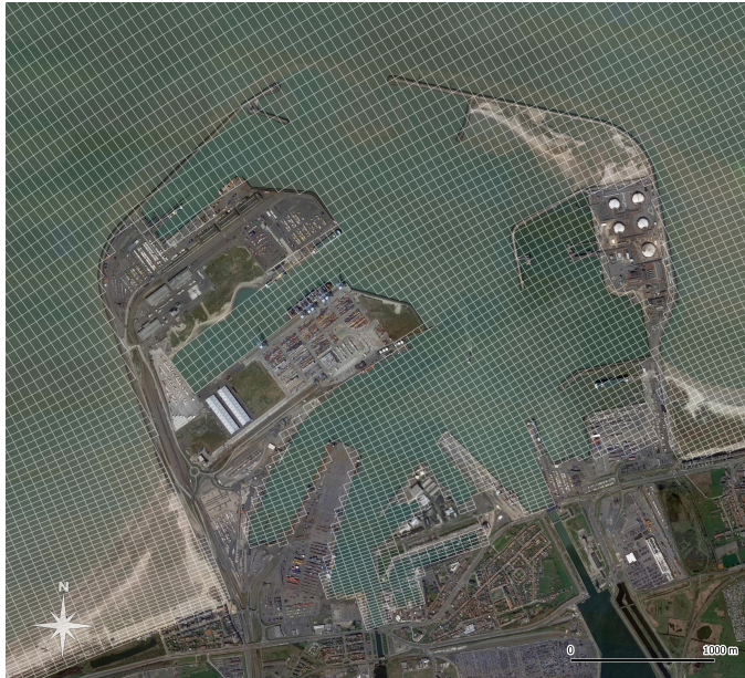
Figure 5.5: Detail of the flow grid in the harbor of Zeebrugge. The background satellite image is from Google Earth.
