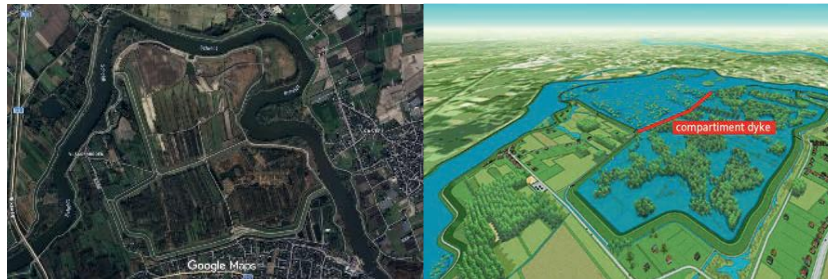
Figure 1.17 Vlassenbroek flood control area: (a) aerial view (Google maps, 2026) and (b) schematic representation of flood control area in function (source: Van Nederkassel et al.,(2015)
