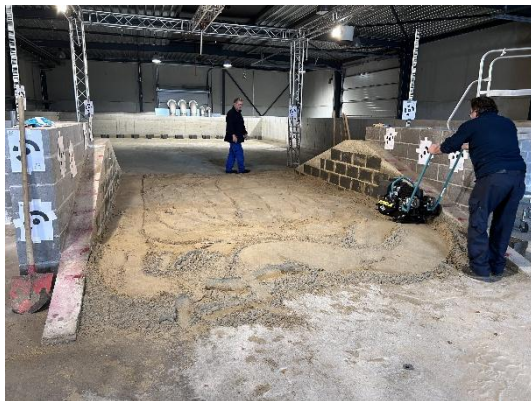
Figure 4.4 Embankment compaction procedure: (a) compacting soil in layers of 0.1 m and (b) vibration plate compactor (Ammann APF-10/33).
