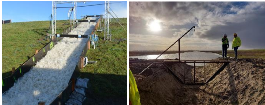
Figure 1.16 Example of field experimentation and emergency response activities: (a) levee overflowing and (b) 'Breachdefender' (source: https://polder2cs.eu/ ).
