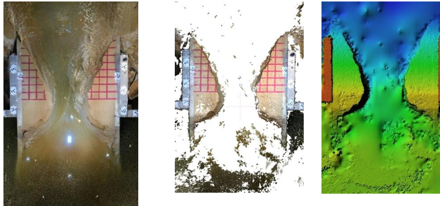
Figure 4.16 Orthophotos, dense point cloud and DEM models at selected moments for test mS_Q_2 , with wood chips supplied at the upstream end of the reservoir.
