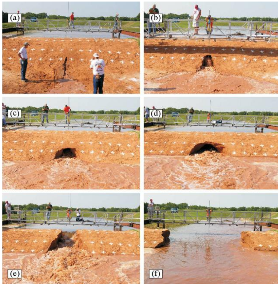
Figure 1.8 Embankment (dam) breaching induced by piping: (a) breach initiation; (b) t=5 min; (c) t=8 min; (d) t=13 min; (e) t=13 min, immediately following the collapse of the pipe roof; and (f) t=60 min, illustrating continued lateral widening. Reprinted from Hanson et al. (2010).
