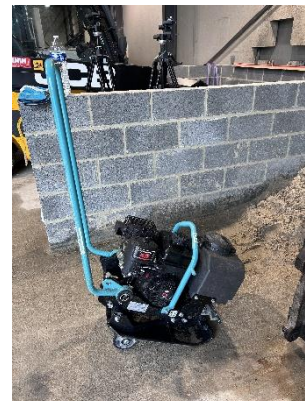
Figure 4.4 Embankment compaction procedure: (a) compacting soil in layers of 0.1 m and (b) vibration plate compactor (Ammann APF-10/33).
