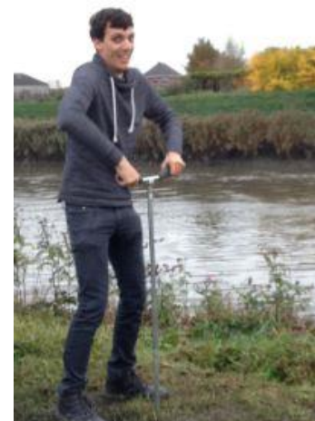
Figure 4-2 Installation of sensors using an auger
