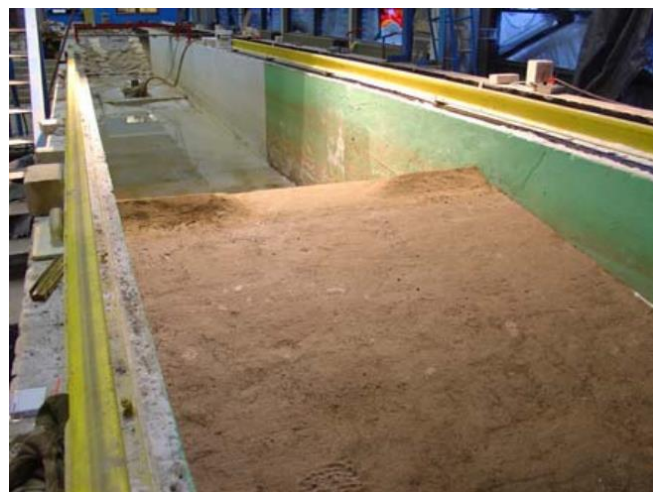
Figure 2-6 Dike model view from seaward side
