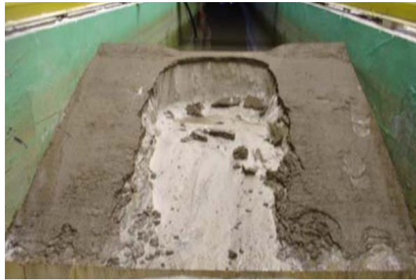
Figure 2-7 Model after breach test (Geisenhainer & Kortenhaus, 2006)
