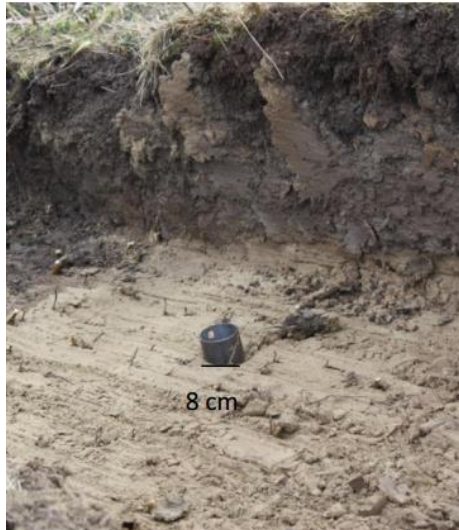
Figure 1-4 clay lining and inner sand core (Irstea, 2015)
