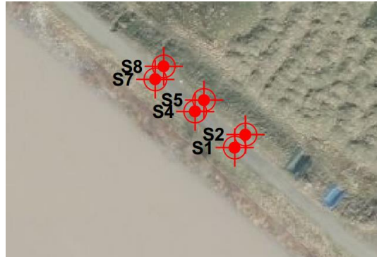
Figure 3-2 CPT-tests on dike crest (DOV, 2016)
