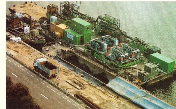
Mechanical test processes for the cleaning and consolidation of dredged silt
