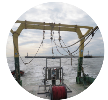
Deploying the Image Sediment Profiler. (© ILVO)
