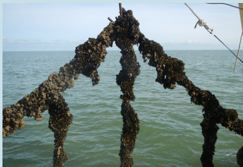
Biobased ropes deployed as mussel droppers at sea being tested on biodegradability. (©ILVO)
