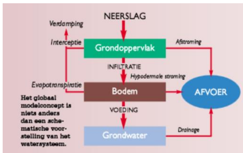
Figuur 7: Globaal modelconcept hydrologisch model (Ecorem-Haecon, 2002)
