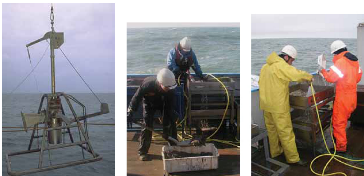
Figure 5. Reineck boxcorer for sampling infauna. Sampling size 0.07 \text{ m}^2 to a depth of 40 cm. Samples are washed over 1 mm sieves.
