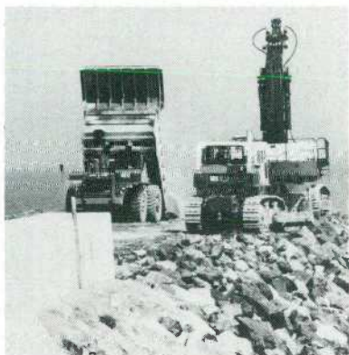
Some of the 10 Aveling Barford 40 ton dump trucks used in building the outer port.
