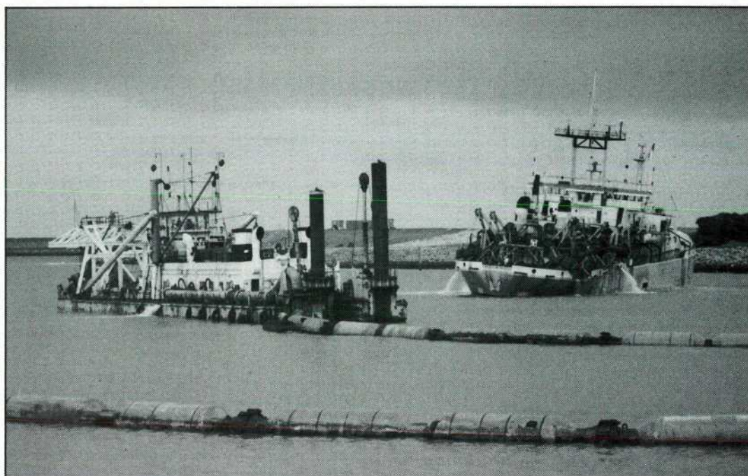
Jan de Nul's trailer-suction hopper dredger "Sanderus" dumping sand for re-dredging and pumping to the western breakwater area by the cutter dredger "Ortelius".
