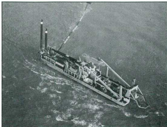
Top: Jan de Nul's self-propelled sea-going cutter suction dredger "Marco Polo" (20,088 hp) at work in protected waters removing bad soil layers under the northern breakwater of the L.N.G. terminal.
