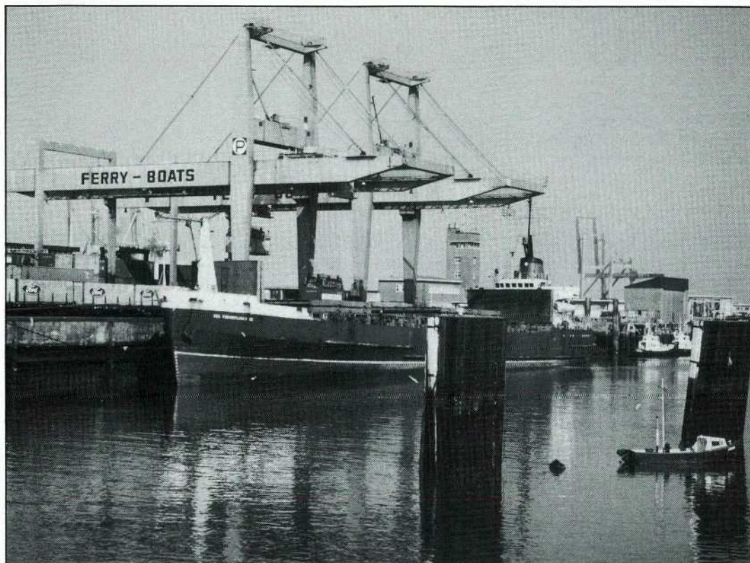
The Shortsea Container Terminal serves the cross-Channel container trade; the facility's two Peiner gantry cranes are pictured here servicing the "Sea Freightliner II".
