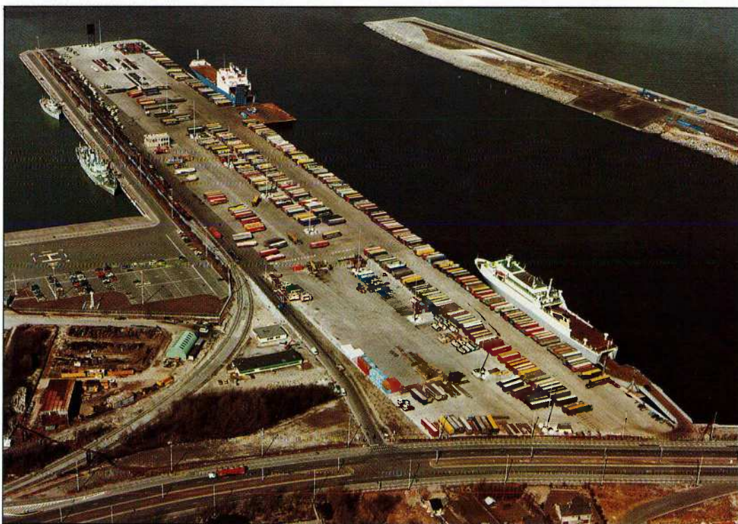
Capacity of Sea-Ro Terminal's Zweedse Kaai facility has recently been improved by installation of a MacGregor-Navire linkspan, seen here in the bottom right-hand corner; the first linkspan has since been re-located to the Westerhoofd.
