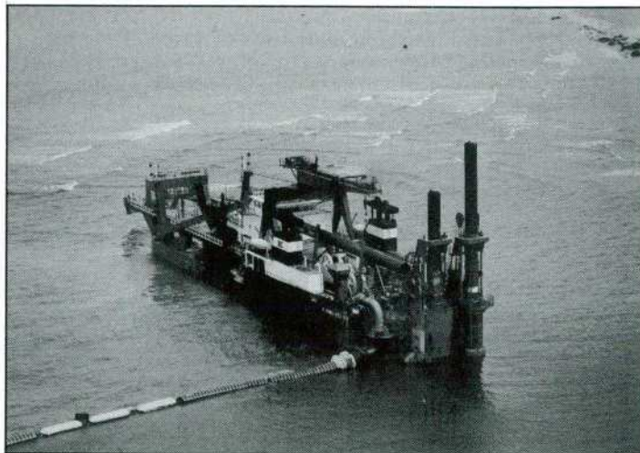
Bottom: Dredging International's trailer-suction hopper dredger "Schelde II" (3,200 \text{m}^3 ) removing bad soil layers in the foundation of the western breakwater.
