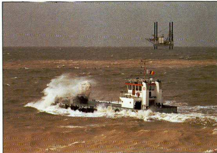
Crew transport to the self-elevating platform "Launcelot" in bad weather conditions; the "Launcelot" was equipped with an NCK heavy duty crane (capacity 80 t at 30 m radius) and two 120 t crawler cranes for compaction.
