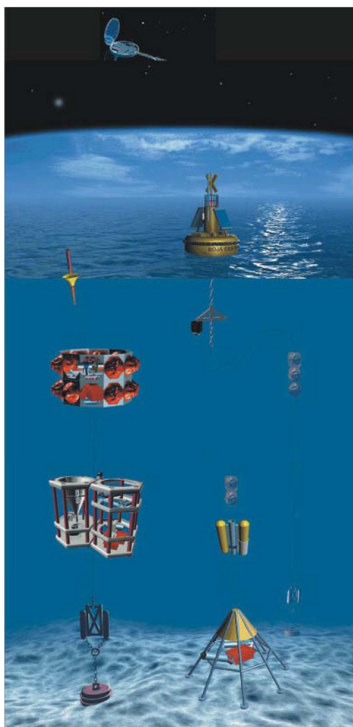
The DOMEST System for observing material transport at the sea bed includes traps, video, profiling CTD and other sensors, with acoustic and satellite retrieval of data using bi-directional communication. © MARUM, Bremen, Germany
