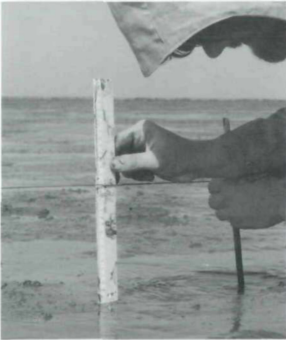
Burying depth of bivalves was measured either with thin nylon threads that were attached on the shell with super glue (left photos), or with a core sampler that was thrust into the mud, after which the core was extracted, placed horizontally and broken carefully (right photos)
