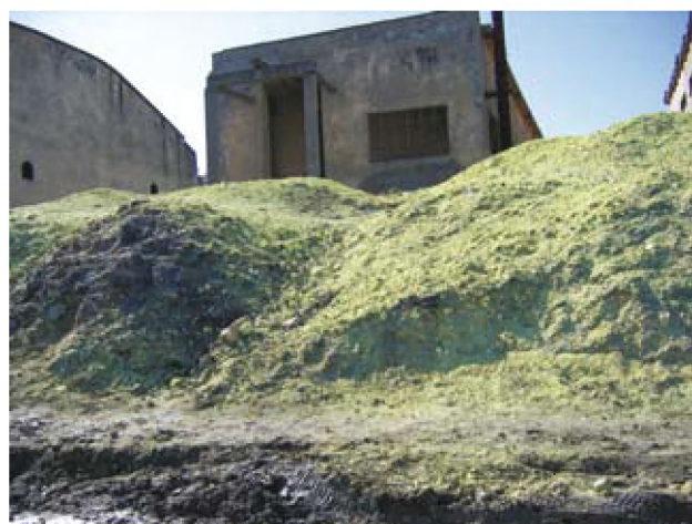
Photo 2.2: Contaminated soil containing sulphur and chromium salts at a closed chemical factory, Porto Romano (Durres, Albania).
