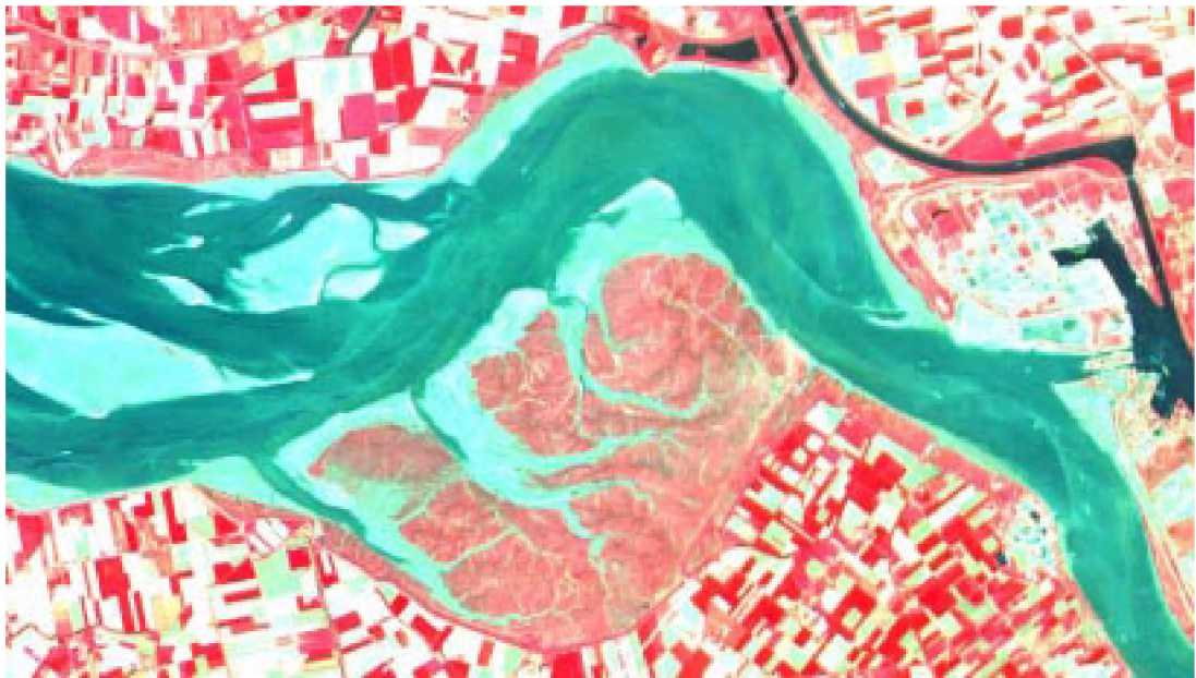
Figure 3.1 False colour composite of SPOT for 10 May 1998 (incoming water, rising tide). The influx of SPM from the Belgium part of the Scheldt can be seen.
