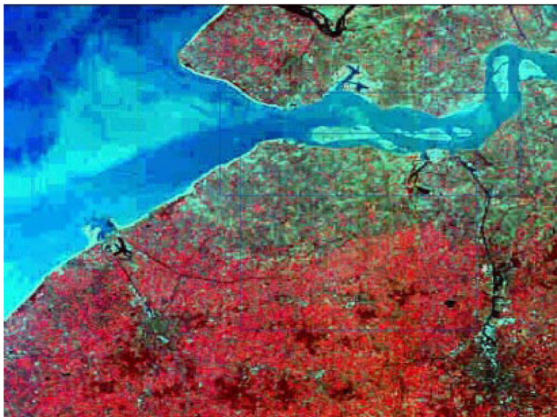
Figure 3.3 SPOT image of 14 February 1998 from Dali Catalogue (~ 11.00 hours; low water). A triangle of high SPM concentration, typical for all winter images is visible at Vlakte van Raan at the mouth of the Western Scheldt.
