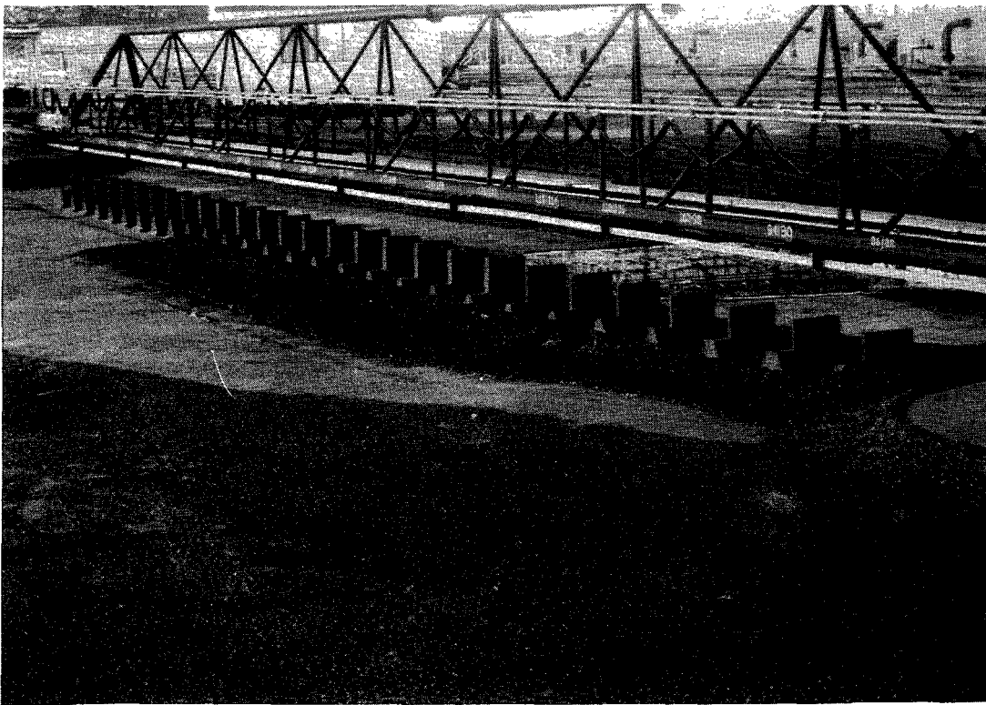
Figure 5.15 View of building stage in the model; placed piers and rubble sill partly completed
