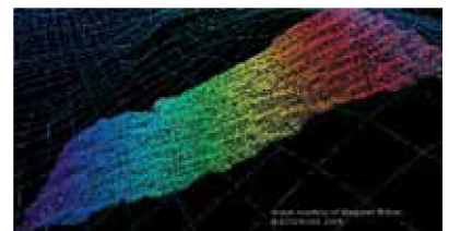
Example of ROV-based multibeam bathymetry data (0.5m grid) with INSS multibeam bathymetry data (25m grid)
