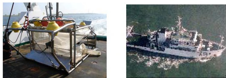
Figure 8.2: Hyperbenthic sledge (left) used for sampling of mysid shrimp in the Scheldt estuary. The sledge was operated from the research vessel Belgica (right).
