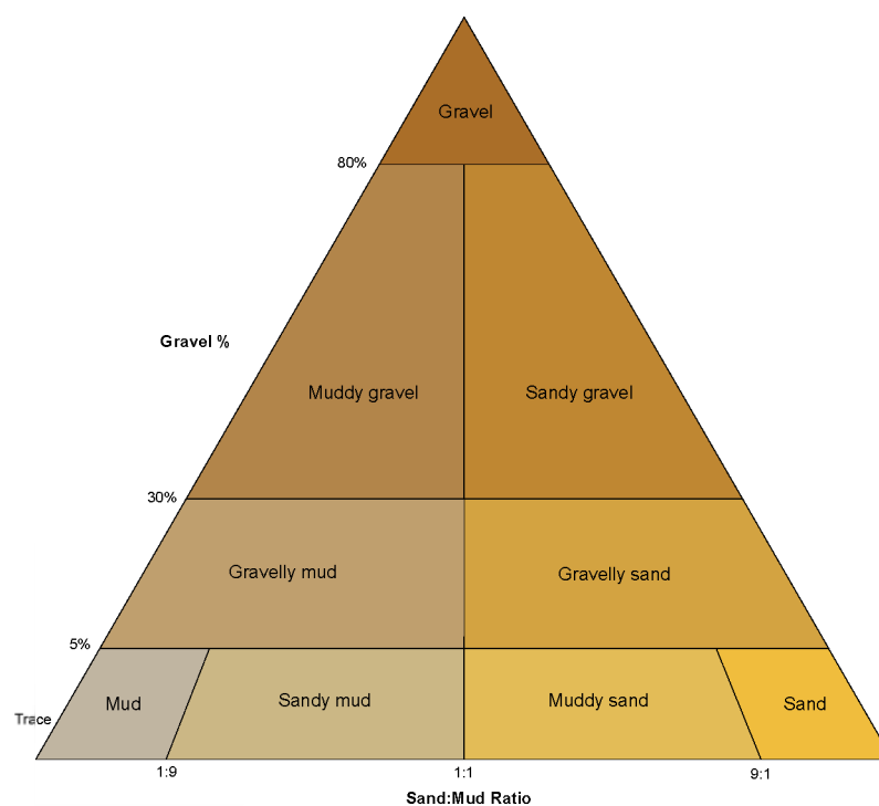
Figure 4.2.1. Standard descriptors of sediment type, according to % particle size contributions (after Folk, 1954).
