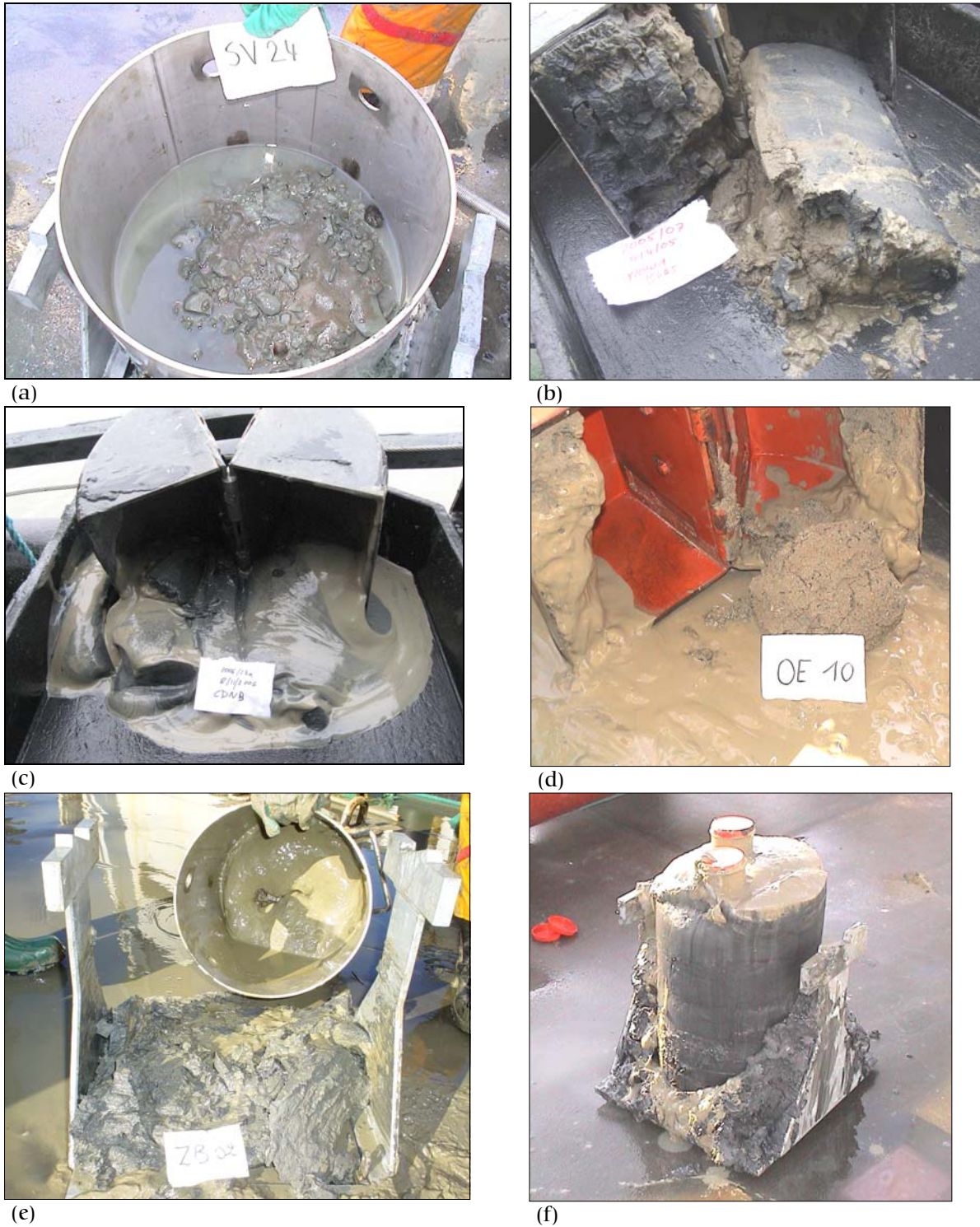
Figure 4.2: Photos of Van Veen (VV) grab (size of grab is 0.3 m × 0.2 m) and box core (BC) samples (height of core is 0.5 m), see Figure 2.1 for geographical location. (a) BC showing mud pebbles on top (SV24, 19/02/2003), the core has been taken near the dumping place B&W-S1; the pebbles could originate from deepening dredging works. (b) VV sample of layered Holocene mud covered by a thin ephemeral sand layer (MOW1, 04/04/2005).
