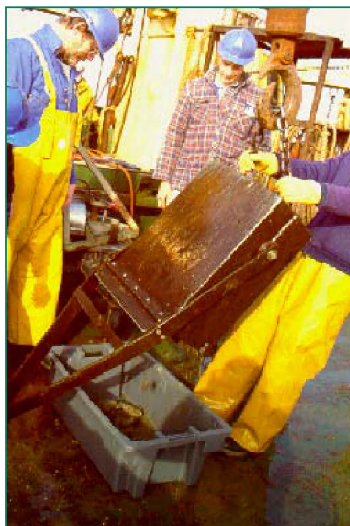
Figure 14 A CEFAS modified Anchor dredge. Note the solid rectangular metal collection box (as opposed to a net bag as in the original design), the open side of which forms the mouth of the dredge. The warp is attached to a hinged wishbone arm which enables the dredge to collect a sample irrespective of which side it lands on the seabed
