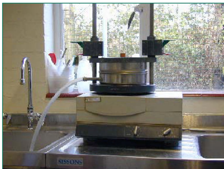
Figure 34 The automated wet sieve shaker is used to split a sediment sample into a coarse fraction and fine fraction. The coarse fraction remains on the sieve, and the fine fraction passes through the sieve to be retained in a collecting pan. The two fractions may then be treated separately for further particle size analysis
