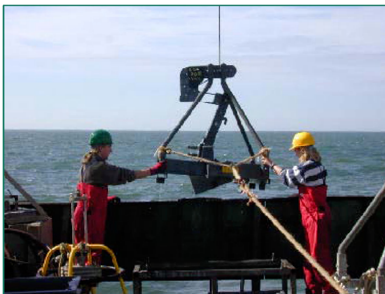
Figure 6 A 0.1 m 2 Hamon Grab being retrieved. Note the use of a winch-controlled lateral supporting rope for increased stability (and therefore safety) during deployment and recovery. It is unhooked before descent of the sampler
