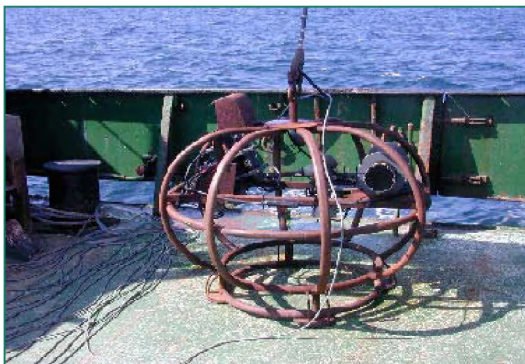
Figure 17 A drop-camera frame. The video and stills cameras, lights and flash unit are housed within the protective metal frame, orientated to collect images of the seabed directly below the frame
