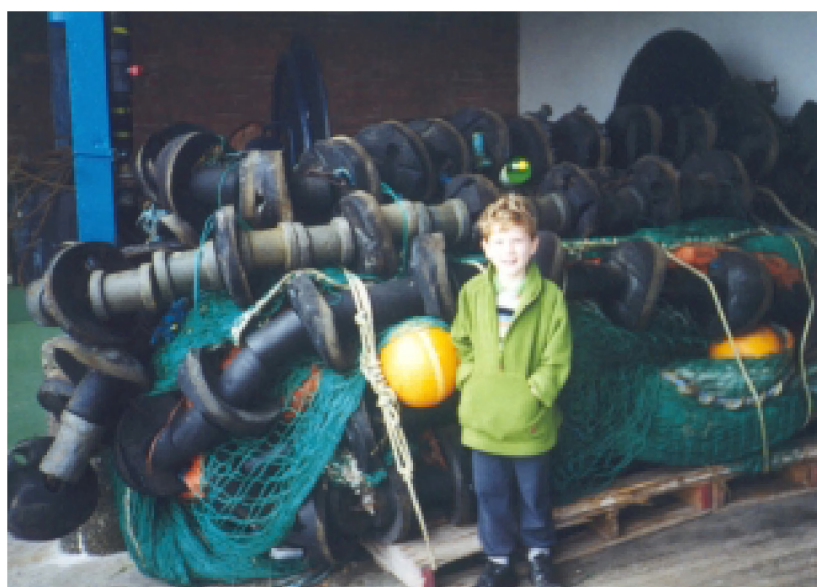
Figure 42. Rockhopper fishing gear developed to fish on previously untrawled rough fishing grounds
