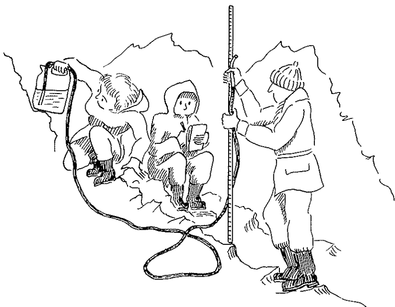
Fig. 2. The use of can and tube for levelling. Providing that the siphon in the tube is unbroken, the water surface in the can and the meniscus at the distant end of the tube must be at the same level. This allows the height of another point to be measured directly as shown.
