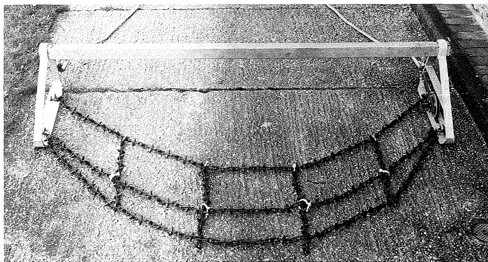
Fig. 1. The standard two-metre beam trawl (a), modified so that the tickler chains are replaced with spiked chain (b, c).
