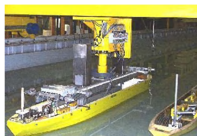
Fig.10 Squat of a containership ( L_{OA} = 291.3 m, B = 40.3 m, T = 13.5 m) sailing at a forward speed of 12 kts, caused by a head-on passing encounter with a bulk carrier ( L_{OA} = 310.6 m, B = 37.8 m, T = 13.5 m) sailing at different forward speeds. Lateral distance between centrelines: 114.5; water depth: 17.1 m. [3]
