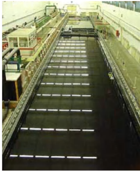
Figure 1. Towing tank for manoeuvres in shallow water.
