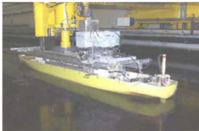
Figure 2. Ship model during captive manoeuvring test.
