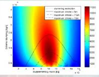
Absorbed power [W] as a function of external damping and supplementary mass with implementation of slamming and stroke limitations for  $H_{\rm s}$  values between 1 and 1.5 m. The buoy is a cone-cylinder with diameter of 4m and draft of 3 m. The area enclosed by the contour lines has to be avoided in order to satisfy the restrictions.
