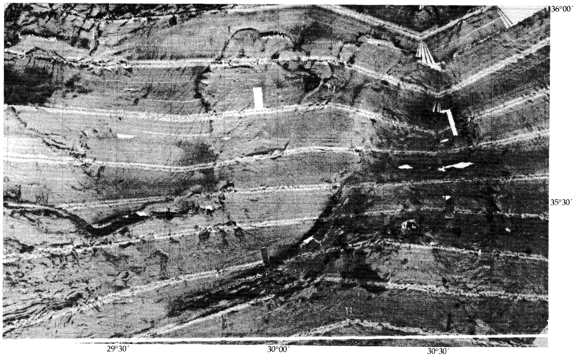
Fig. 8. Simrad EM-12D seafloor reflectivity imagery of the Anaximander Mountains (Woodside, 1995). Dark shades indicate high reflectivity and lighter shades lower reflectivity. The ship's track is highlighted by a lighter shaded strip in the centre of each swath of data
