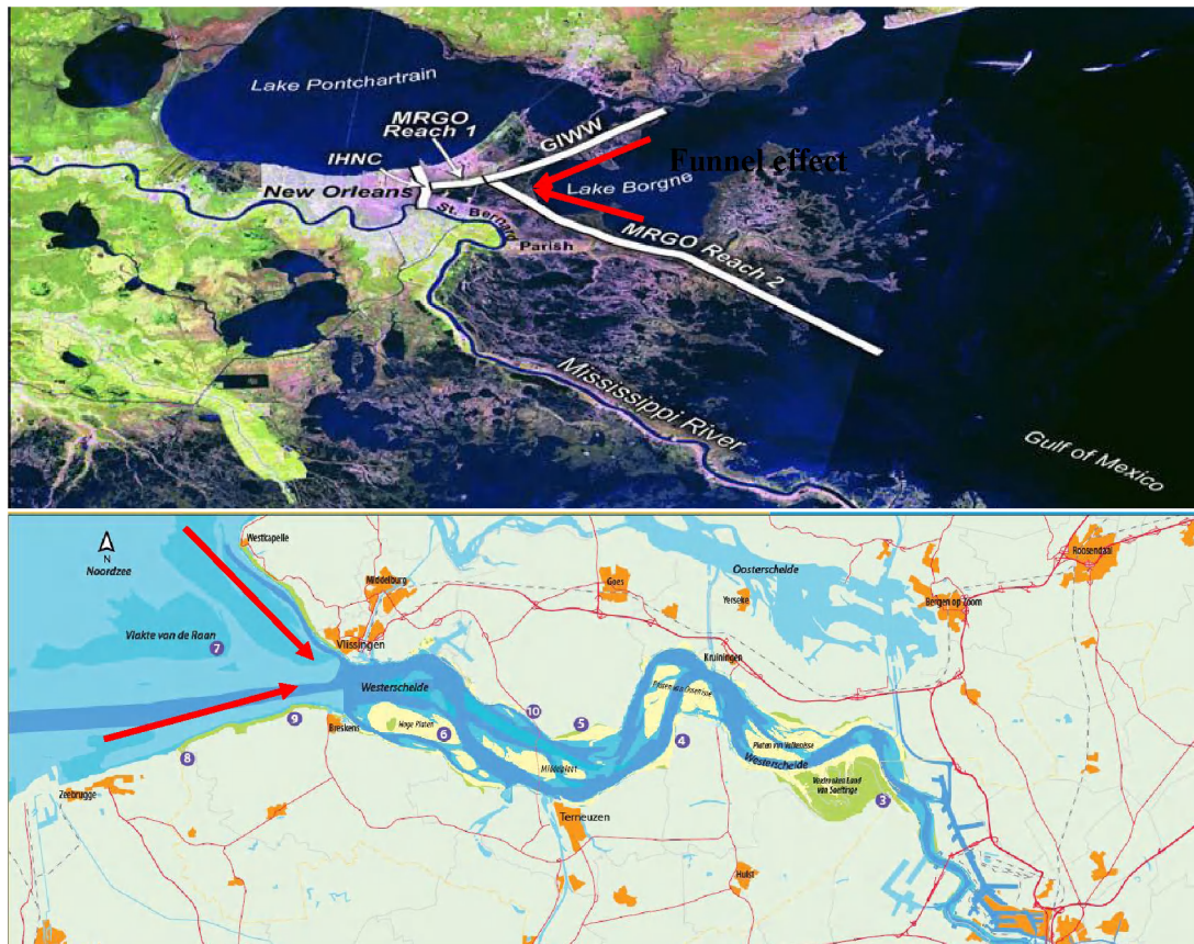
Figure 14 Funnel effect that may enhance the storm surge levels (source top picture: Carter N T and Stern C V, 2006).
