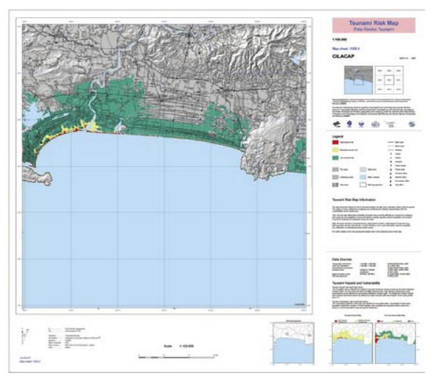
Fig. 6.1 Tsunami risk map at a local scale
