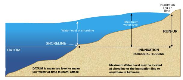
**Fig. 3.1** Tsunami impact at the coast: an explanation of terms.
