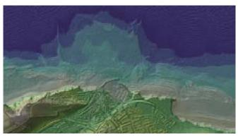
**Fig. 4.1**. LIDAR digital surface model for coastal terrain and nearshore seabed mapping This example, showing bathymetric zonation and seabed morphology, is from Watchet in England, United Kingdom
