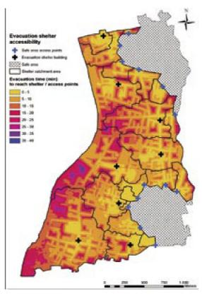
**Fig. 7.3** Evacuation map for Kuta, Bali. Map shows the time in minutes (short time=yellow; long time=red, purple) people need to evacuate to vertical shelter buildings or horizontal shelter areas. Source: GITEWS Project. Courtesy DLR.
