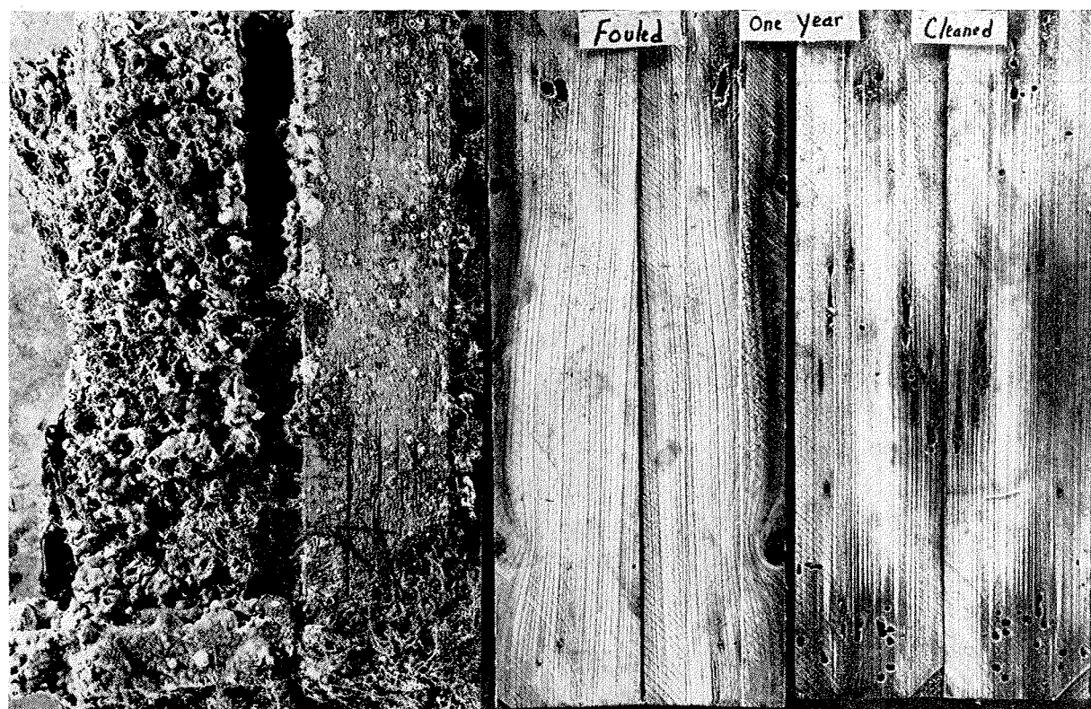
FIGURE 22. Effect of fouling on attack by wood borers. Fouling on the block at left was undisturbed during one year's immersion at Miami Beach. The block at its right was cleaned periodically to reduce fouling. The condition of the blocks when split open is shown at right.
