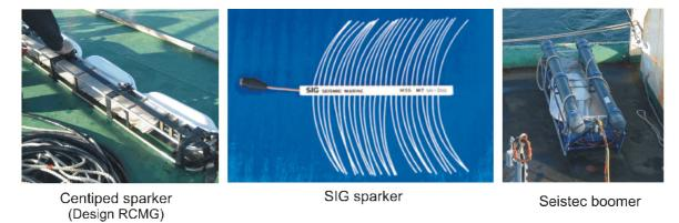
Fig. 3.2 Overview of the seismic sources applied during the recent surveys (1990-2007). For technical specifications see Table 3.2.
