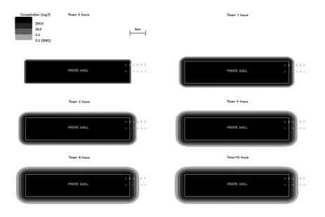
A shell leaking over its entire surface was located at a depth beneath the sediments of 0.2 m.
