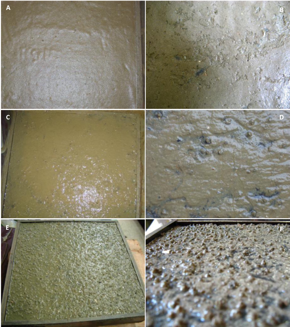
Figure 2: Pictures showing different density treatments before and after erosion. A: Control before erosion, B: Detail of control after erosion with visible erosion of thin sediment flakes, C: 4,000 ind./m 2 before erosion, D: Detail of 4,000 ind./m 2 after erosion with local erosion around the burrows, E: 20,000 ind./m 2 before erosion and F: Detail of 20,000 ind./m 2 after erosion with protruding burrows and visibly eroded sediment between the burrows.
