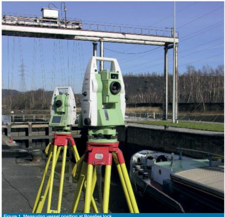
Figure 1. Measuring vessel position at Rose
