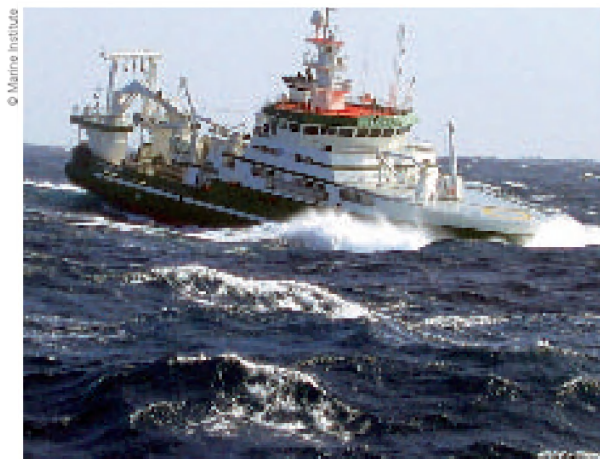
Figure 14. The Irish Marine Institute's Research Vessel Celtic Explorer is the national platform for offshore Marine Research. She is 65.5 m in length and accommodates 31 personnel, including 17-19 scientists
