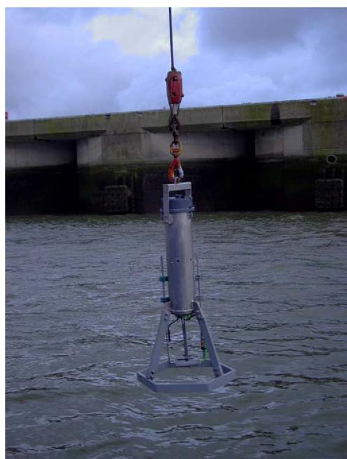
Figure 2-5: High Resolution SiltProfiler
