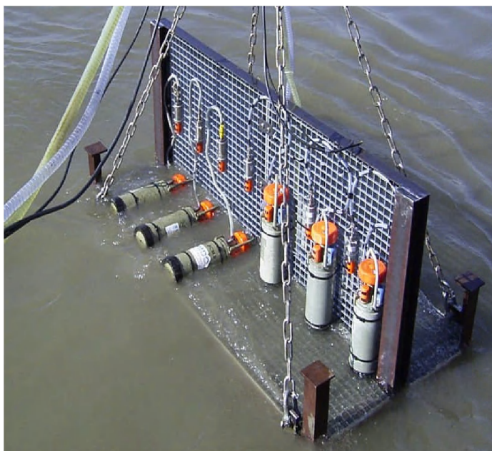
Figure 2-1: Calibration frame with double pump set-up
