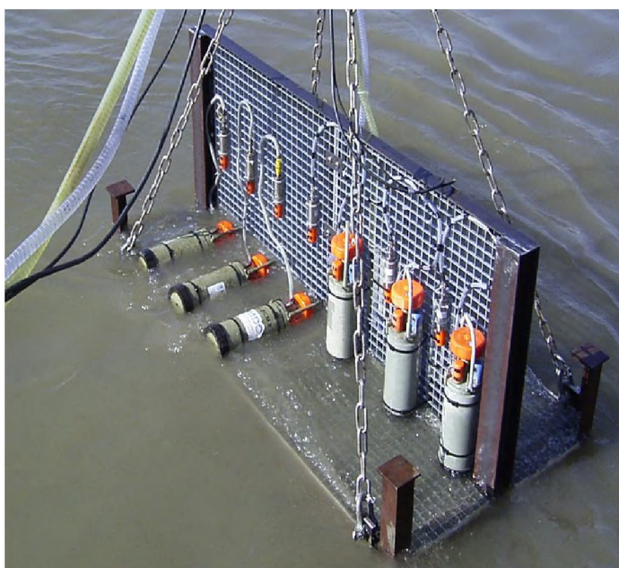
Figure 2-1: Calibration frame with double pump set-up
