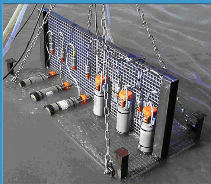
Calibration Frame set-up (left) & Measurement locations (right)
